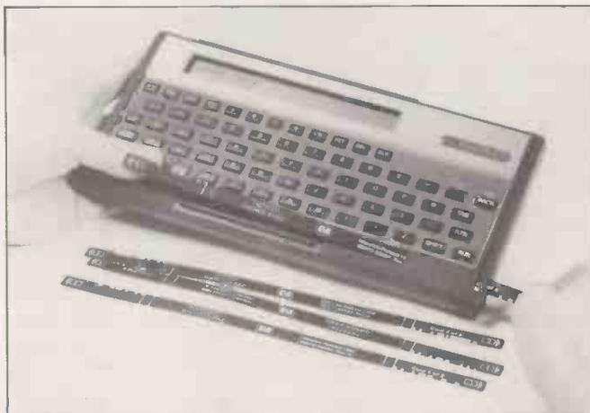
ware defined to customise the machine to a particular application, and provision is made to accept clip-on keyboard overlays. There are three slots beneath the lower edge of the keyboard for 16K plug-in ROM modules, which could neatly hold the customising applications software.
